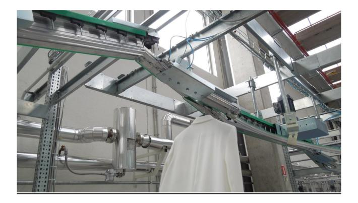
Made of aluminum profile, the pin transporter, on one side has a chain roll installed and moved by gearbox, on the other side a special steel profile to support the plastic contour, in order to process a better flow of the hangers.
