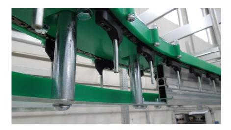
The internal transporting conveyor is used for hanging garments, trolley or different products less than 40kg.
